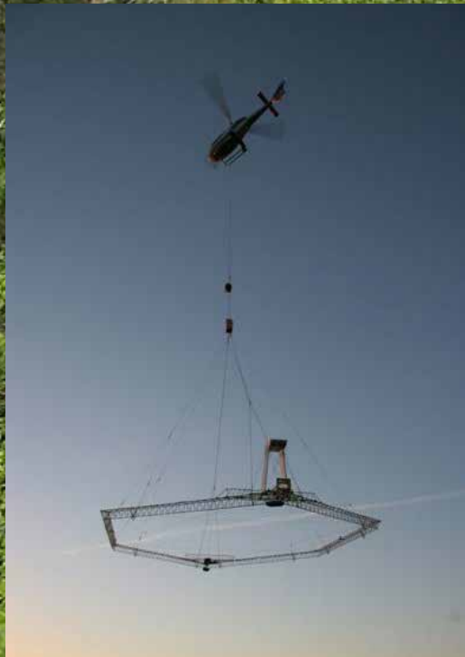
Regional mapping, Malaysia New technology makes it possible to map water and minerals from the air. In Southeast Asia, in Malaysia, airborne technology has been used for very large geophysical surveys of groundwater. These involved flying over 15,000 kilometres (9,000 miles) in 30-40 kilometres (18-25 miles) long parallel tracks, covering an area of 3,000 square kilometres (1,100 square miles). Several Danish companies worked together in order to carry out drilling, down hole logging, water-quality testing, well field design, geological and hydrological modelling. The survey revealed a potential source of 500 million litres of groundwater per day (130 million US gallons). (Courtesy: SkyTEM Surveys and EnviDan International)
